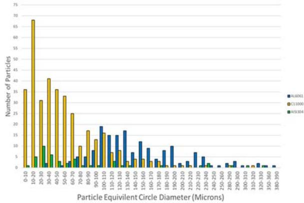
**Figure 7: Measured Size and Number of Particles from Arc Test Ejected Molten Metal Material**
