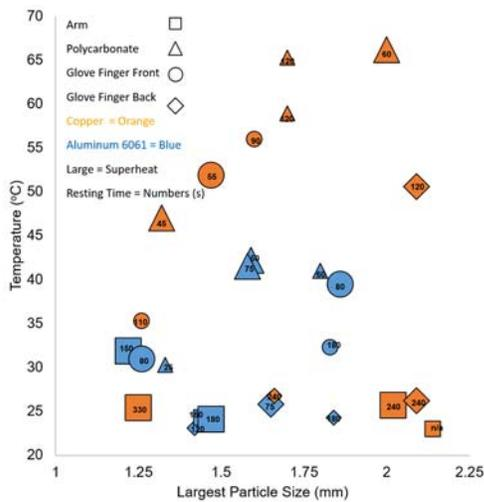
**Fig. 12: Backside Temperature vs. Largest Particle Size (Particle Break-up Method).**
