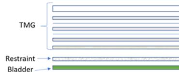
Figure 2: Glove Finger Back Cross-Section
