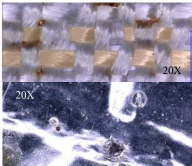
**Figure 15: TMG Shell Molten Metal Seepage and MLI Damage**
