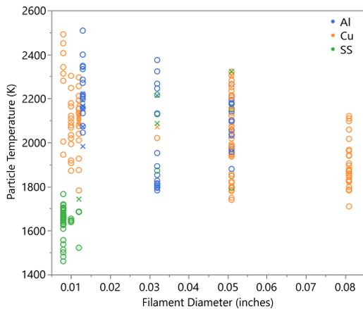
**Figure 5: Measured Particle Temperatures from Arc Test Ejected Molten Metal Material**
