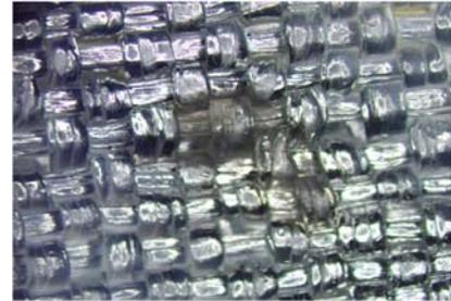
**Figure 13: Metal Vapor Deposition on TMG Shell Material (20X)**
