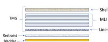
Figure 1: Lower Arm Cross-Section
