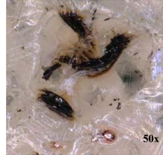
**Figure 17: Entrapped Ejecta and Damage to TMG Palm Material**
