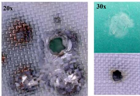
**Figure 16: Burn Through Damage to Glove Finger Back TMG Shell and Restraint Materials with Thermal**
