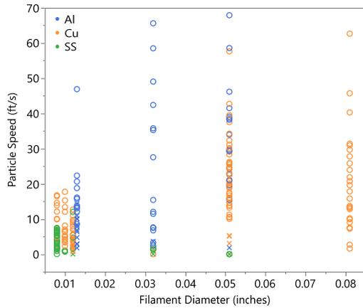
**Figure 6: Measured Particle Velocities from Arc Test Ejected Molten Metal Material.**
