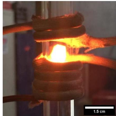
**Figure 8: Hot Metal Levitating in a Magnetic Field**
