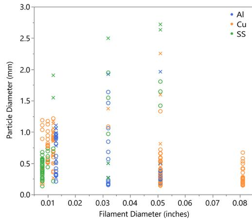
**Figure 4: Measured Particle Sizes from Arc Test Ejected Molten Metal Material.**
