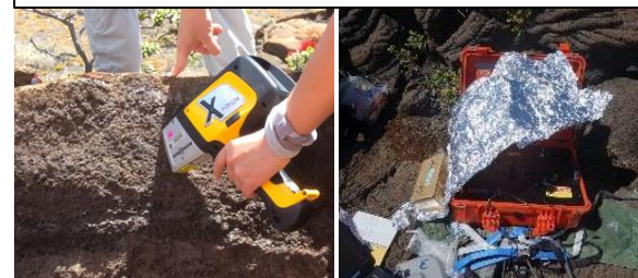
hXRF & XRD for in situ chemistry and mineralogy
