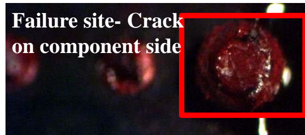
(b) Failure on component side
