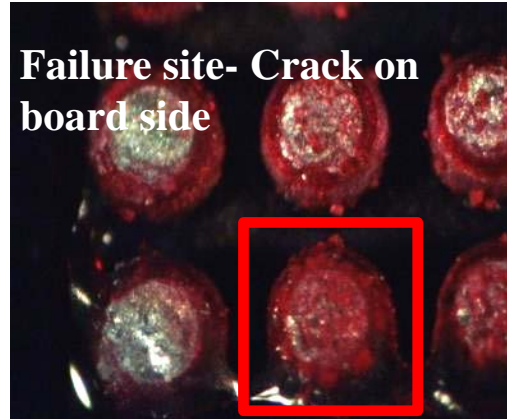
(a) Failure on board side
