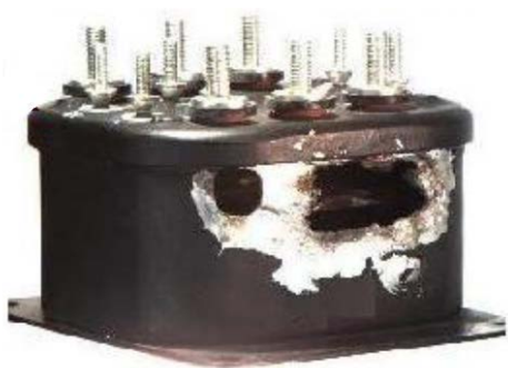
Failed relay due to tin vapor arcing
