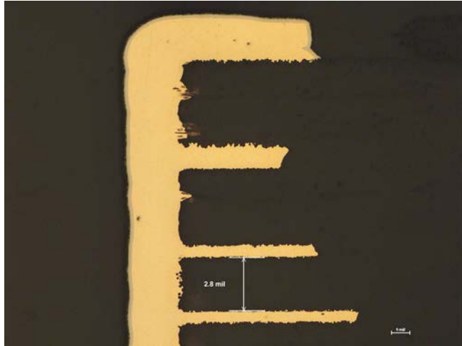
Dielectric layer less than 3.0 mil
