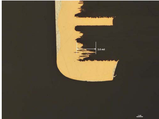
Copper wicking in excess of 2.0 mil
