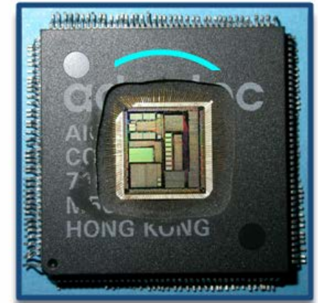
1x Magnification: After Decapsulation*
