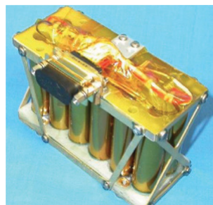
Li-Ion batteries flown on NASA Missions: Mars Exploration, Rover, and the Lunar Reconnaissance Orbiter.
