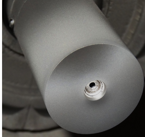
Figure 2.—Photograph of the discharge cathode within EM3 shortly after the ion optics were removed.
