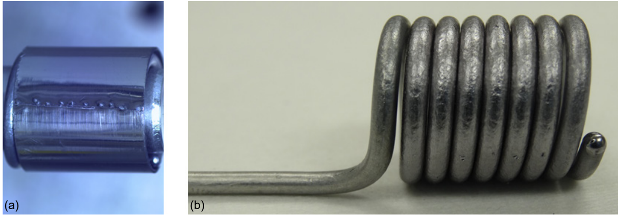
Figure 9.—Photographs of (a) the DCA heater radiation shield and (b) the heater coil after removal from the cathode tube. No visible wear or defects were found to be caused by cathode operation.
