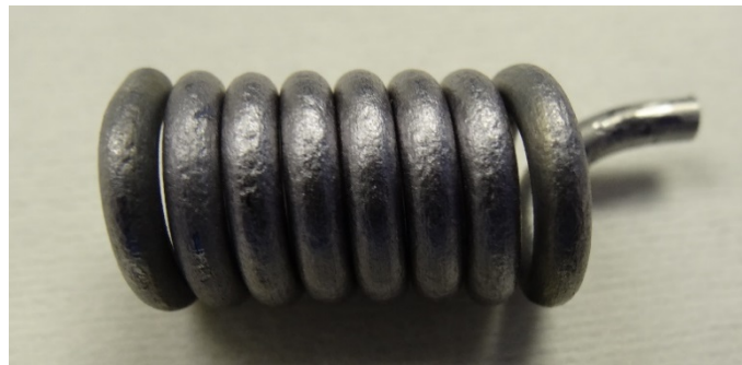
Figure 20.—Photograph of the heater coil after removal from the neutralizer cathode tube. Aside from texturing on the downstream face, the coil was found to be in excellent condition.
