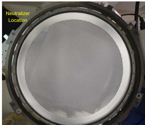
Figure 3.—Post-test upstream screen grid mounted to the ion optics assembly. The orientation of the neutralizer is shown.
