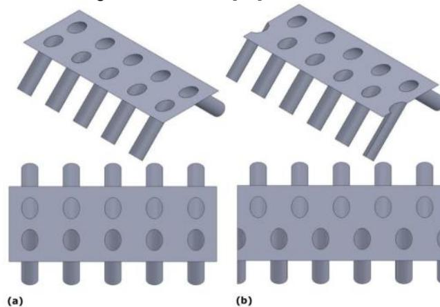
Figure 12. a) Aligned impingement injector element scheme, b) non-impinging and misaligned injector element scheme [24].
