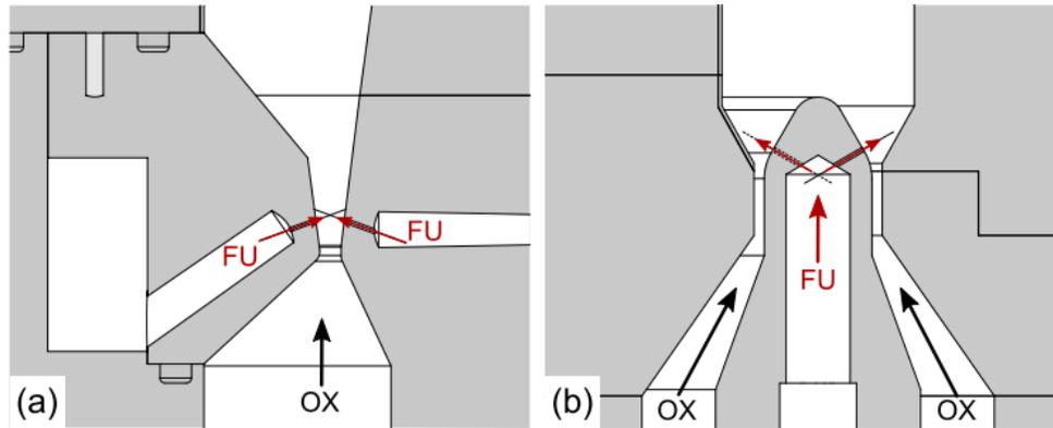
**Figure 9. a) Axial slot injector and b) axial sting injector from [11].**
