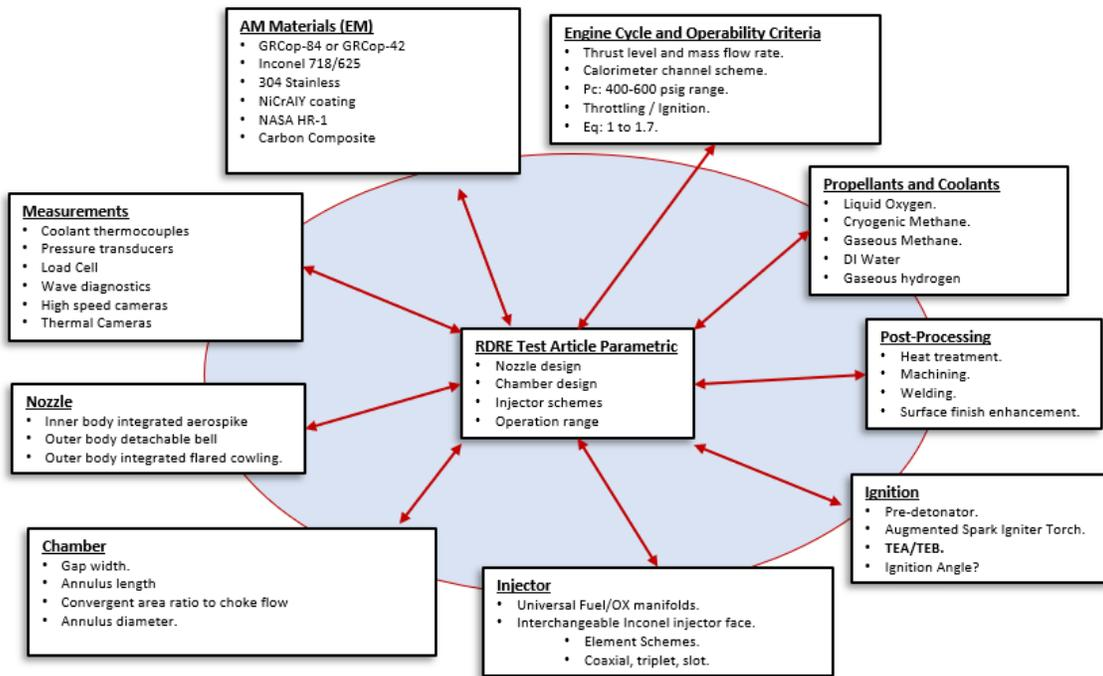
**Figure 6. Consideration diagram for development of an optimized performance RDRE.**
