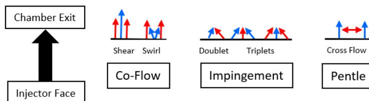
**Figure 22. Traditionally manufactured injector element orifice flow vector relative to the axial chamber coordinate system.**
