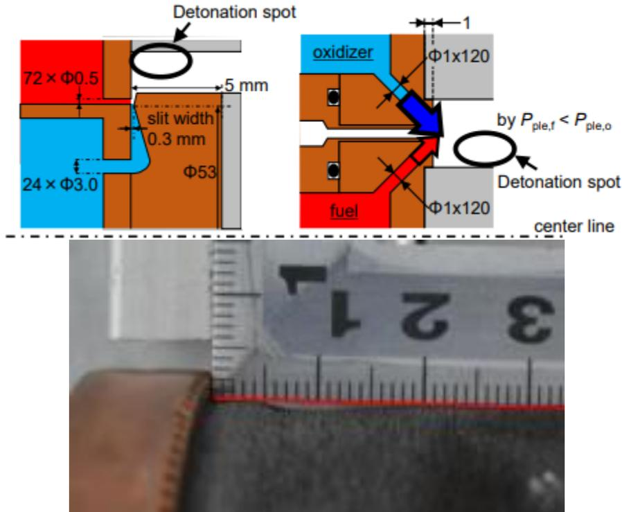
**Figure 15. Injector element schemes tested under [26] (top) and region of anchored detonation causing damage to the chamber carbon composite wall using the triplet configuration.**
