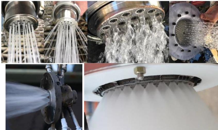
**Figure 20. Water flow testing of various thrust class AM injectors.**
