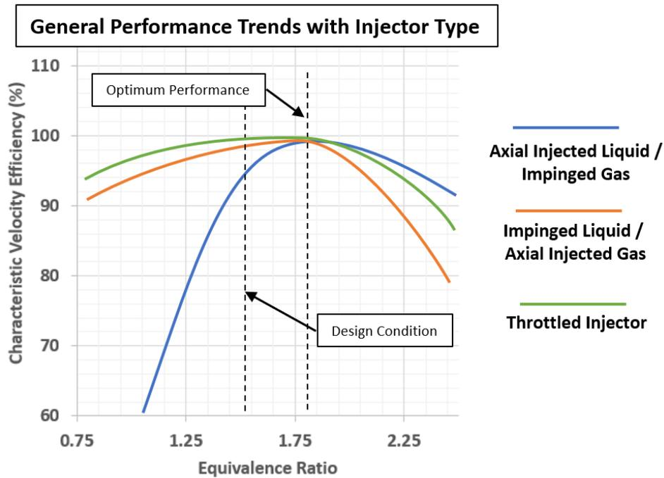
**Figure 23. General performance trends of traditionally manufactured injector elements.**
