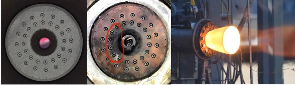
**Figure 4. JBK-75 additively manufactured shear coaxial injector. (Left) Prior to testing under PJ141 and PK020. (Middle) Post-testing with More than 3130 seconds of cumulative duration and 21 starts over 2 test series in LOX/GH2 at a nominal Pc of 1000 psi and mixture ratio of close to stoichiometric. Slight face erosion shown in the red circle but not deleterious to injector operation. (Right) Hot fire test demonstration with NASA carbon composite nozzle.**
