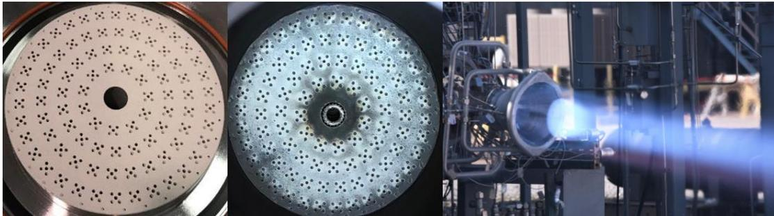
**Figure 5. Inconel 625 L-PBF 7K lbf class pentad impinging injector face. (Left) pre-hot fire testing with NiCrAlY thermal barrier. (Middle) More than 720 seconds of cumulative hot fire duration and greater than 32 starts in LOX/GCH4 at a nominal Pc of 750 psi and mixture ratios up to 3.6. (Right) Hot fire test demonstration of AM impinging injector, L-PBF GRCop-42 chamber, and LP-DED NASA HR-1 regenerative nozzle.**
