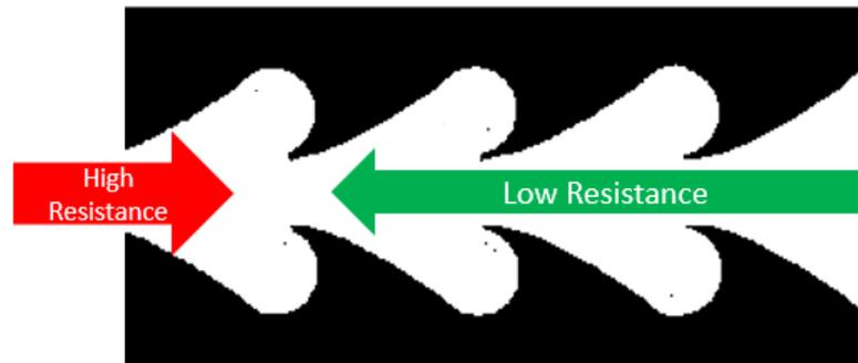
**Figure 24. Tesla type fluid diode with high resistance in the reverse direction and low resistance in the forward direction. Individual junctions or cavities also shown.**
