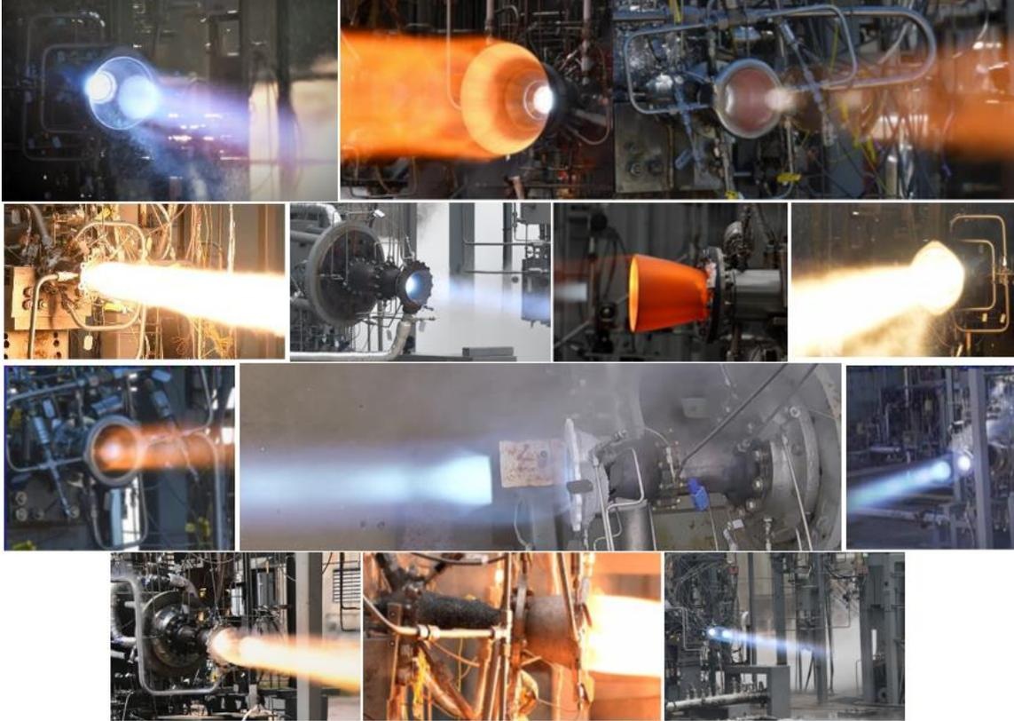
**Figure 1. Hot fire testing of metal additively manufactured thrust chamber assemblies including additive injectors, chambers, igniters, and nozzles in various propellant combinations and thrust classes.**
