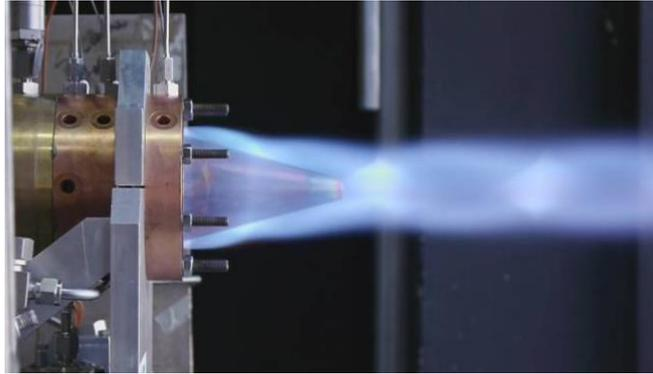
**Figure 13. AFRL GHKN RDRE during hot fire test [24].**
