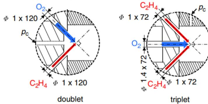
**Figure 14. Injector element configurations tested under the experimental investigation in [25].**
