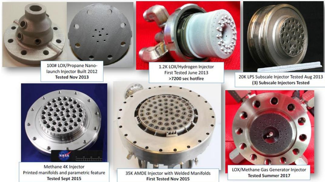
**Figure 19. Various L-PBF Injectors manufactured and tested at NASA MSFC.**
