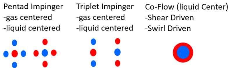
**Figure 16. Traditionally manufactured and most common liquid bi-propellant injector elements schemes. Blue represents liquid phase propellants and red represents gas phase propellants.**
