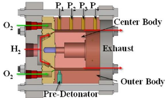
Figure 11. RDRE test article hot fire tested in [23].
