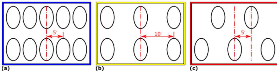
**Figure 8. Impinging injector element schemes a) aligned 72 element pairs ~0.131” spacing, b) 36 element pairs ~0.262” spacing, c) misaligned 36 element pairs ~0.131” spacing [20].**
