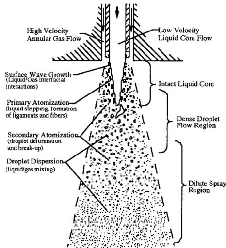
Figure 17 Coaxial injector element and atomization spray field [30].
