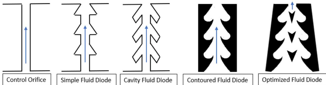
**Figure 25. Potential fluidic diode structures integrated into an injector orifice and control case for comparison.**
