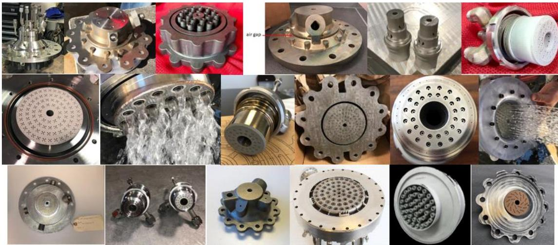
**Figure 3. Examples of various thrust class and material metal additively manufactured liquid rocket injectors hot fire tested at NASA MSFC.**
