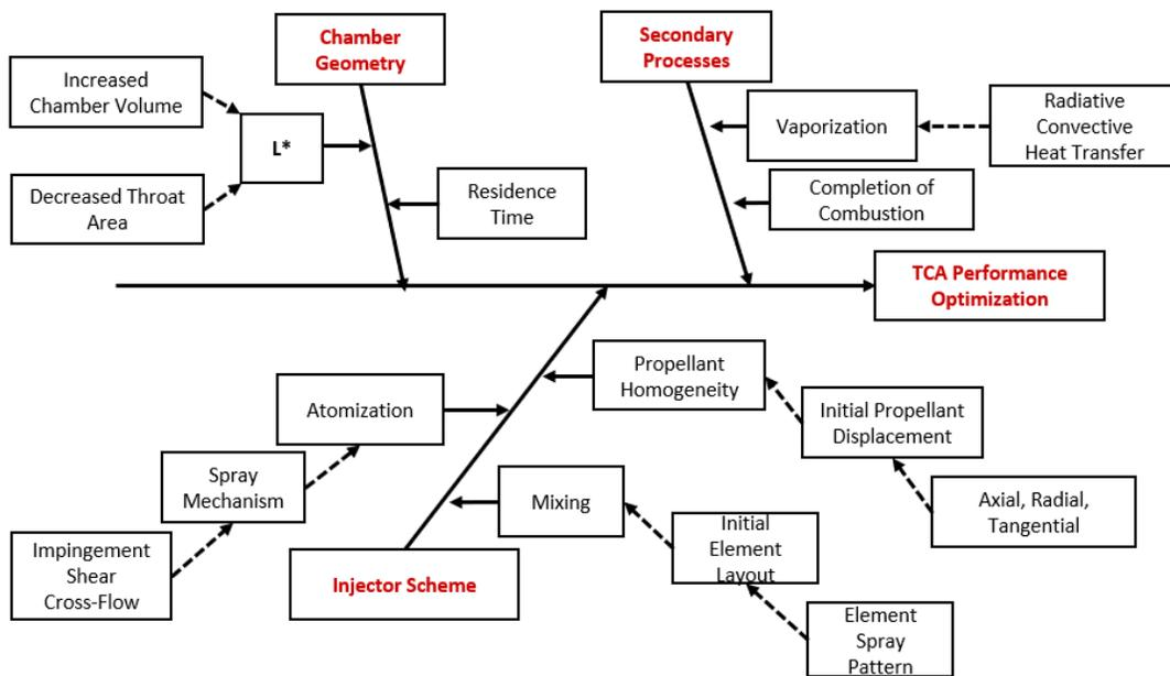
**Figure 18. Process flow diagram for considerations in combustion performance of an injector assembly.**
