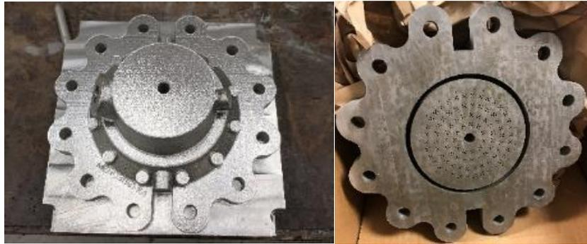
**Figure 21. NASA 7K lbf LOX/methane pentad impingement Inconel 718 injector.**
