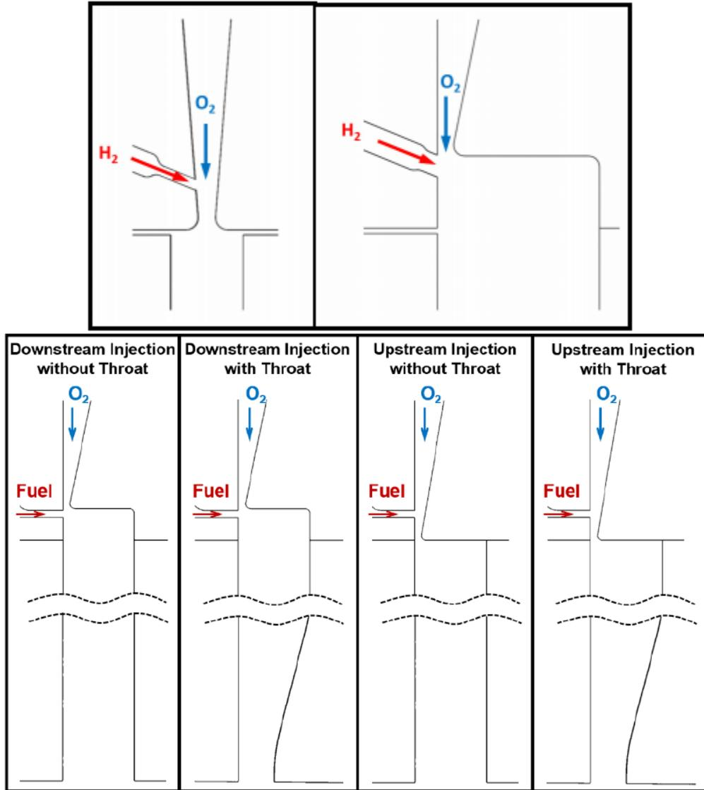
Figure 10. Arrangement of injector and channel schemes experimentally investigated in (Stechmann, et al., 2017). On top left is V1.0 configuration, top right is the V1.1 configuration, and on the bottom are various V1.2 configurations [16].
