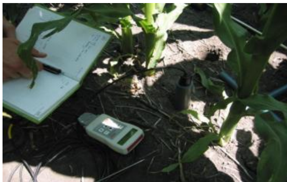
Figure 24: Coincident to gravimetric methods, impedance probe measurements help to improve efficiency of sampling on the ground.
