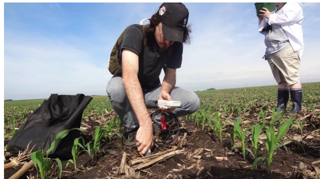
Figure 24: Coincident to gravimetric methods, impedance probe measurements help to improve efficiency of sampling on the ground.
