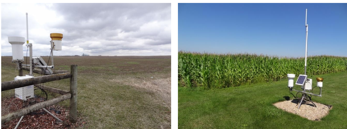
Figure 26: Two examples of in situ network locations which monitor soil moisture as well as soil temperature, and precipitation. Both have sensors buried in soil outside of the station footprint.
