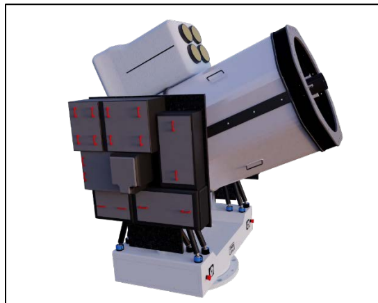
Figure 6. Conceptual rendering of the LCOT telescope with side-mounted optical benches and transmit optical telescope assembly attached.
