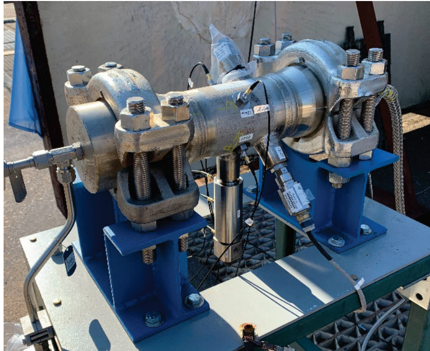
Figure 2. Photograph of high pressure test chamber with pulse gun and instrumentation installed.
