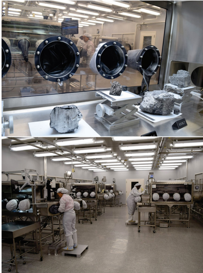
Figure 7: (top) A view of four large Apollo samples on display in the Pristine Apollo Sample Processing Laboratory at Johnson Space Center (left to right samples are 60015,1; 15016,0; 61016,7; and 15459,0). All pristine lunar samples are processed in stainless steel glove boxes using only stainless steel, aluminum, or Teflon tools in an ultra-pure dry N 2 gas environment. (bottom) A view of Apollo sample processors Andrea Mosie (right) and Charis Krysher (left) working in the Pristine Apollo Sample Processing Laboratory at NASA Johnson Space Center.
