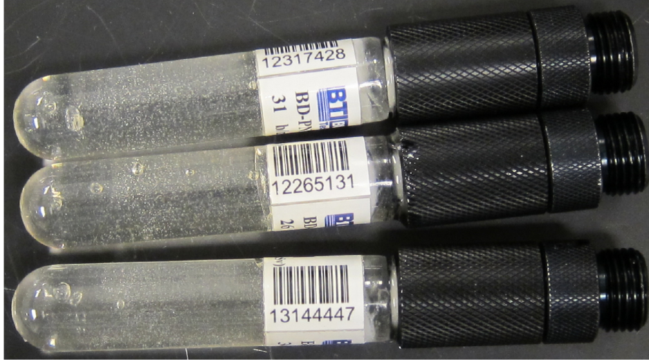
Figure 8.—Bubble detector personal neutron dosimeters. Neutron-induced bubbles are visible in these three uncapped and used bubble detectors. Polymer detection media is translucent section to left of white label, which displays serial number and calibration data for each detector.
