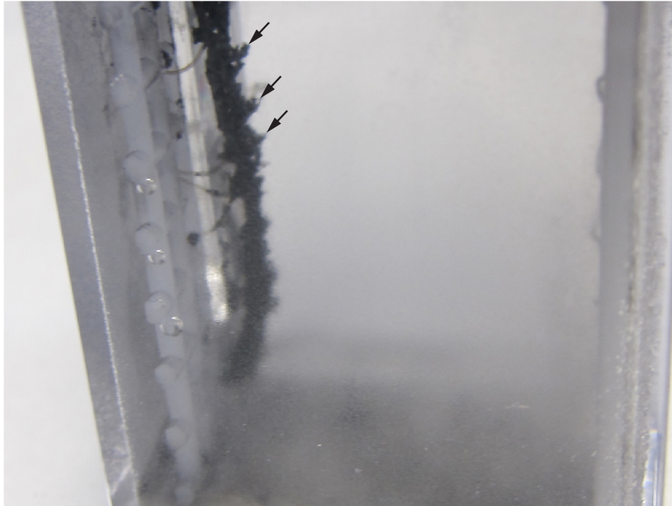
Figure 19.—Dendritic structure on the cathode surface of the best performing experimental cell (T-III-E1).
