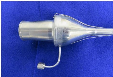
Fig. 3. Stirling hot end integrated into heat pipe condenser
