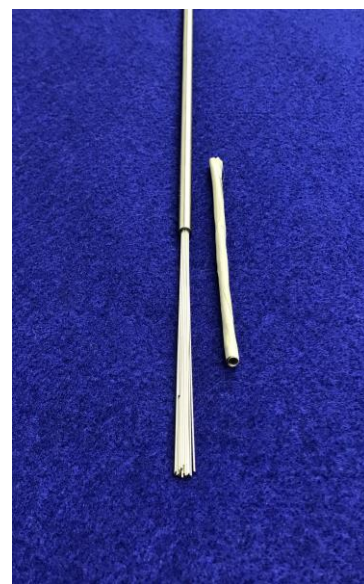
Fig. 1. Examples of capillary tubing and metal screen artery
