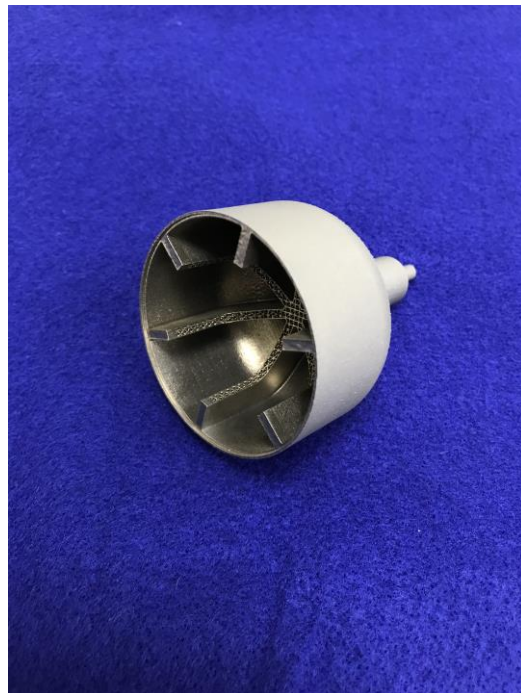
Fig. 4. Additively manufactured heat pipe condenser
