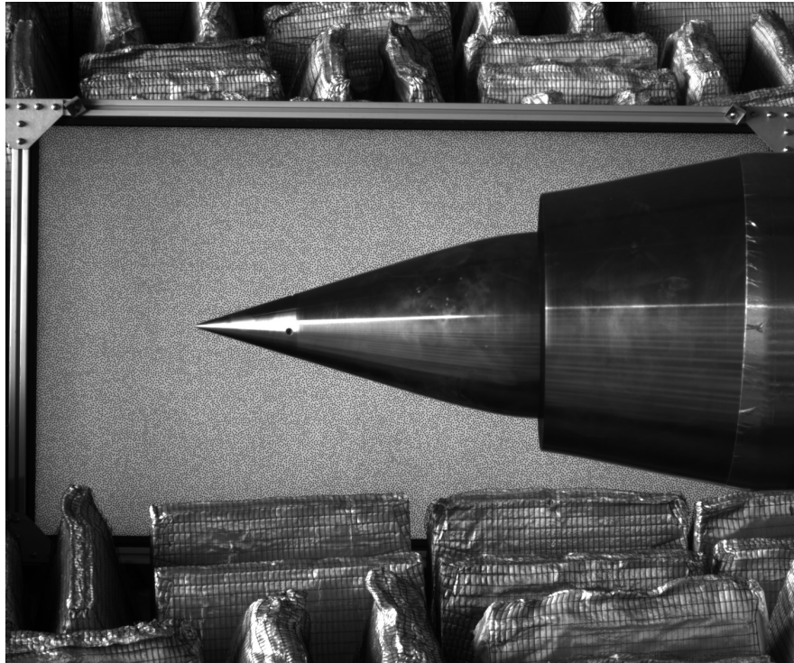
Figure 20.—Raw BOS image showing background speckle pattern. The model is 20 ft away from the background.
