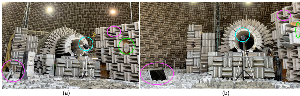
Figure 24.—Diagnostic speakerball test to measure reflections from instrumentation. Speakerball circled in blue BOS camera and monitor circled in pink, phased array circled in green. In photo (a), BOS monitor is covered by a portable wedge wall while the phased array is uncovered. In (b), the BOS monitor is uncovered while the phased array is covered by wedges strapped in front of it.
