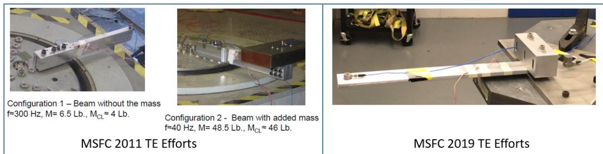
Figure 1: Free Vibration Test Articles and Setup
