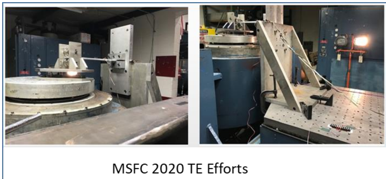
Figure 2: Forced Vibration Test Article and Setup
