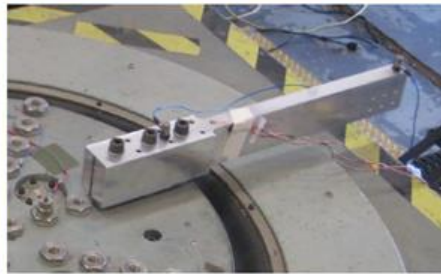
Configuration 1 – Beam without the mass f \approx 300 Hz, M = 6.5 Lb., M_{CL} \approx 4 Lb.
