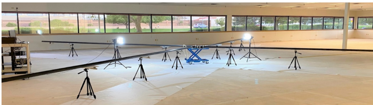
Four one-quarter scale composite booms built and deployed from a prototype sail deployer.
