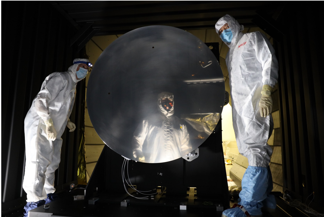
Team members in the MSFC X-Ray and Cryogenic Facility (XRCF). Pictured left to right: Ron Eng, Tomasz Lis (reflected in the mirror's surface), and Ernest Wright. The XRCF is capable of characterizing the cryogenic performance of large mirrors to temperatures as low 30K. (Image Credit: Mark T. Stahl, NASA MSFC)
