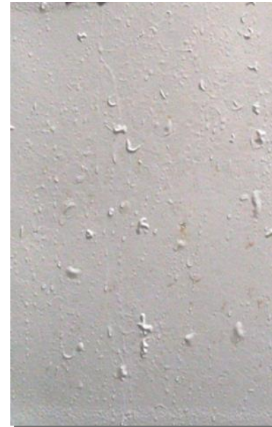
Blistering of Acrylic Topcoat over Inorganic Zinc
