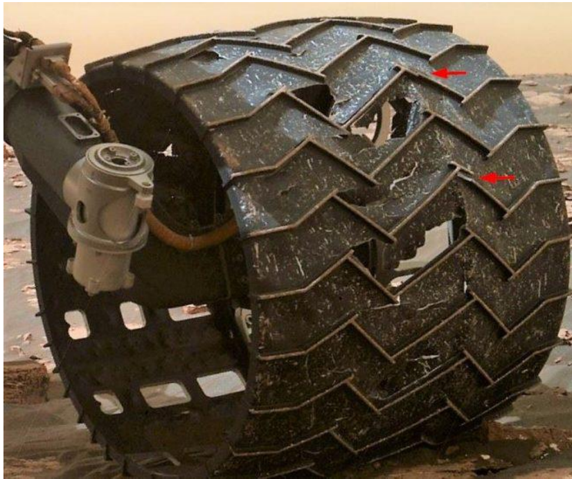
Curiosity rover's wheel, March 19, 2017 (16 km since August 2012)
