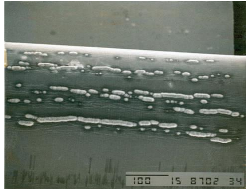
Silver covered with gold where you see the formation of silver oxide caused by atomic oxygen in coating defects
