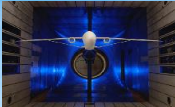
Transonic Truss-Braced Wing 5-10% fuel burn benefit
