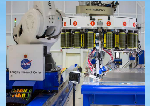
High-Rate Composite Manufacturing 4x-6x manufacturing rate increase
