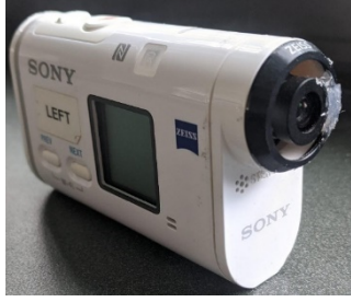
Fig. 6 Sony Action Camera with 8.25 mm lens. The hot glue on the enclosure secured the focus.
