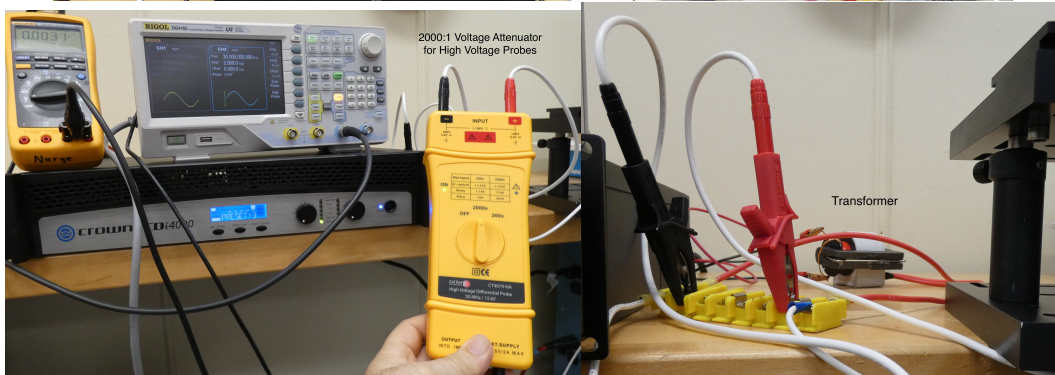
Figure 26. Photos showing test configuration using a step-up transformer to generate the high voltages between the sphere and the ground plane.
