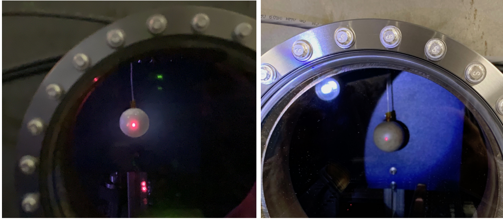
Figure 33. The photo on the left shows the charged sphere in the presence of the plasma. The glow of a corona discharge is present. The bright spots on the sphere are believed to be electrons punching through the paint to try and neutralize the charge. The photo on the right shows the discoloration to the sphere from the hot spots in the paint that occur from the plasma electrons attempting to neutralize the potential.
