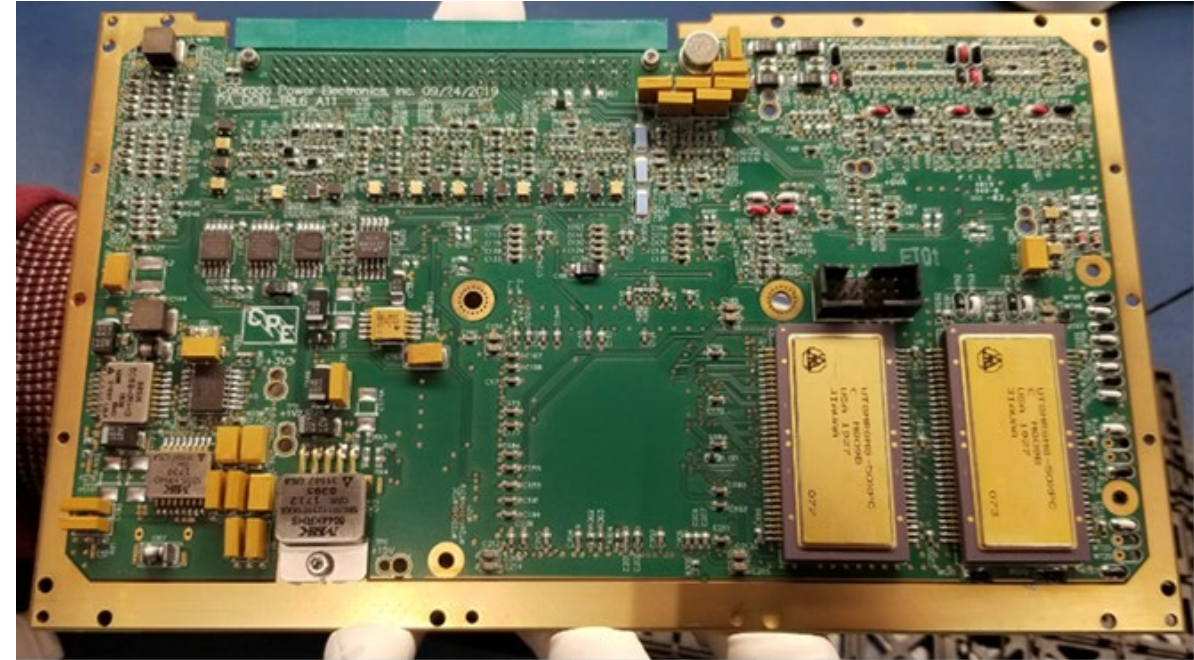
PDU DCIU board with MCM installed
