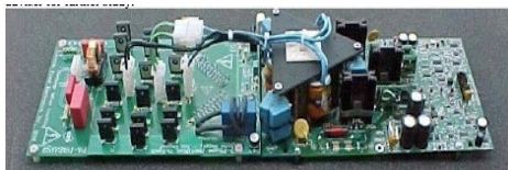
1-kW Breadboard Discharge Module
