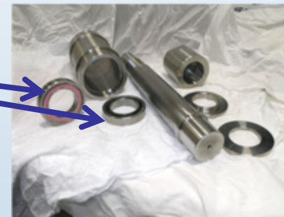
DA Centrifuge Bearing Test Rig Spindle Components
