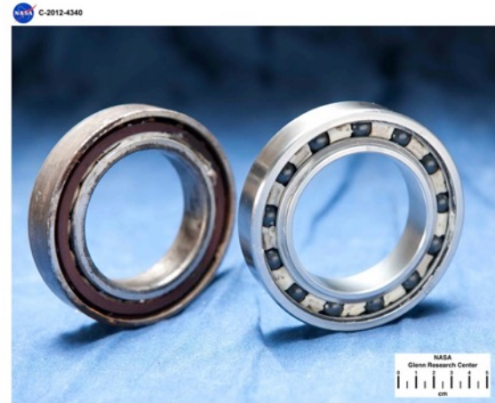
Steel Bearing (rust)
