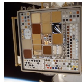
NASA Image: ISS015E19091 – This image of the MISSE-3 Tray 1 Passive Experiment Container (PEC) was taken in July 2007. At this point, MISSE-3 has been exposed to the space environment for approximately 11 months.
