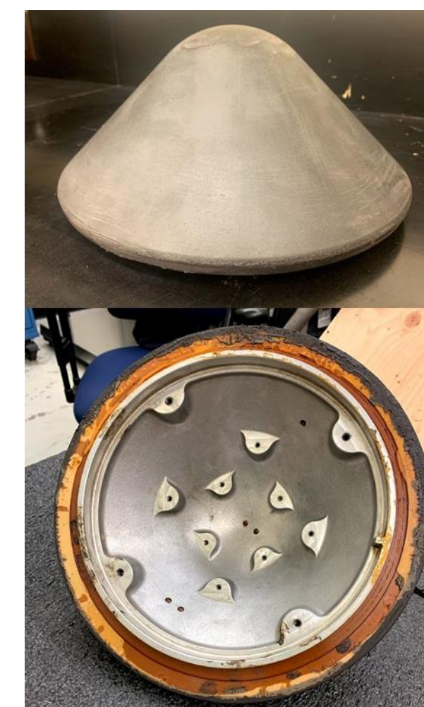
Heat shield after machining. Graded material shown.
