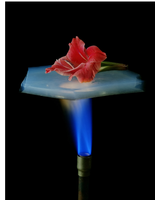
Bunsen burner applied to aerogel (LANL)
