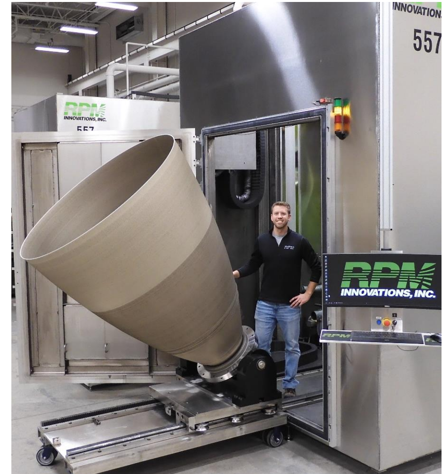
60" (1.52 m) diameter and 70" (1.78 m) height 90 day deposition
