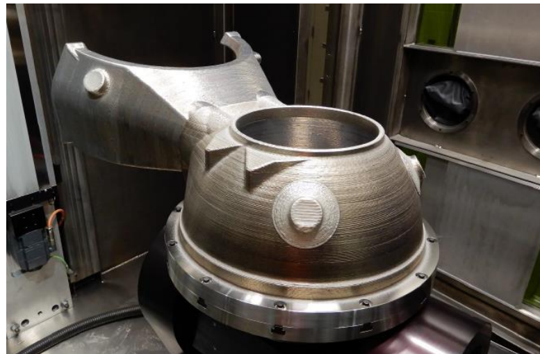
RS25 Powerhead demonstrator using LP-DED under NASA SLS Artemis Program (Courtesy: RPMI)
