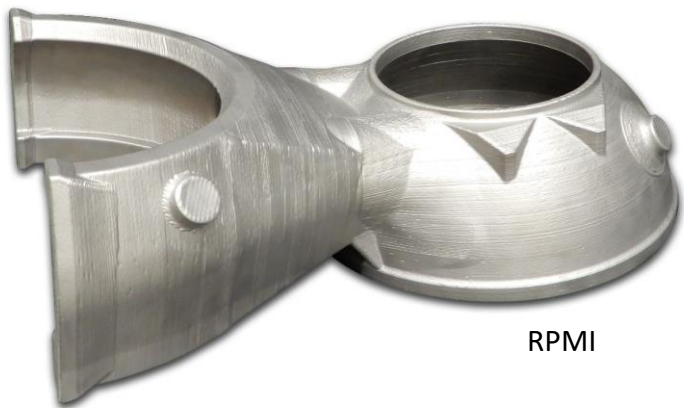
Multi-material combination with L-PBF and DED (RAMPT Project)
