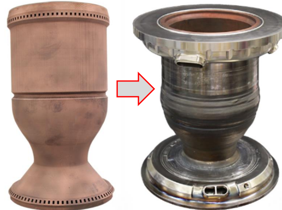
EB-DED Inco 625 Jacket on L-PBF GRCop-84 Liner
