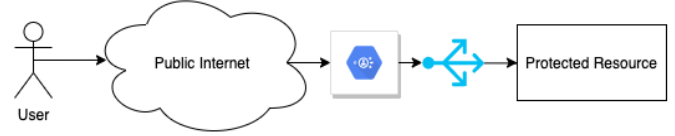
Fig. 2. Architectural flow diagram for IAP terminated ahead of Load Balancer
