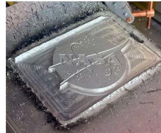
*Example of part produced with Vulcan (prior to substrate removal). Image from Made in Space.*
