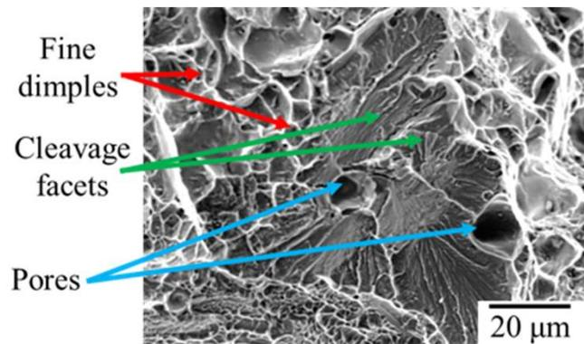
*Fine powder samples exhibit brittle fracture with surface dominated by cleavage facets.*
