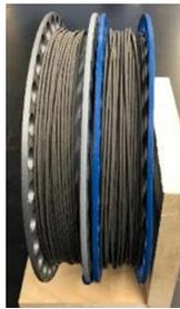
Ti-6Al-4V spooled filament (59% solid loading)
