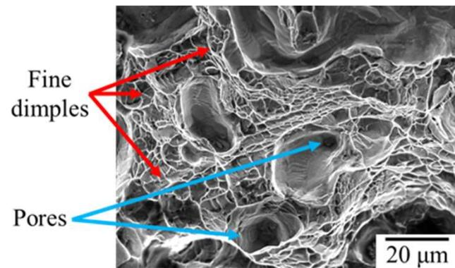
*Coarse powder samples show ductile fracture with the presence of fine dimples.*
