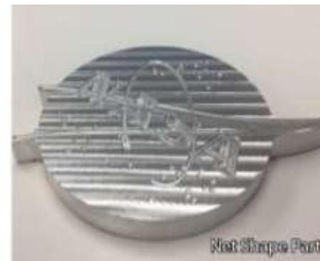
*Steps in the Vulcan hybrid AM process: additive manufacturing via WAAM, subtractive manufacturing, and net shape part. Image from Made in Space.*
