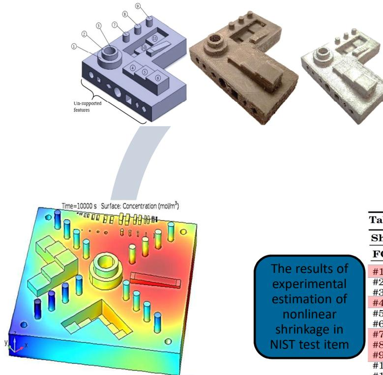
Example of nonlinear shrinkage for NIST standard item manufactured using bound metal additive manufacturing.
