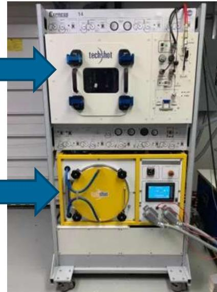
*Ground based prototype system for bound metal additive manufacturing developed by Techshot, Inc. Image from Techshot, Inc.*
