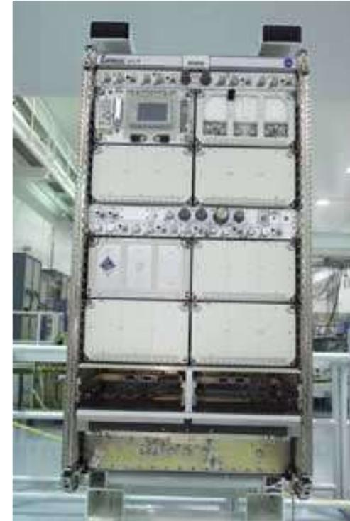
*Image of an EXPedite the PROcessing of Experiments to Space Station (EXPRESS) Rack for ISS payloads. Image from NASA.*
