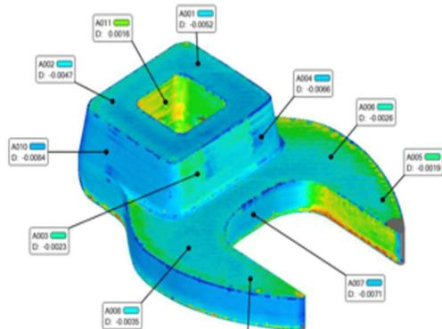
*Structured light scan from NASA Marshall Space Flight Center of crowfoot tool additively manufactured on-orbit. Colors represent deviations from the dimensions in the part file.*
