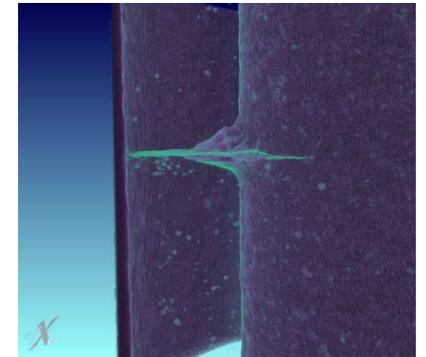
*Future in-space computed tomography (CT) capabilities could provide both dimensional verification and volumetric inspection, including crack detection. X-ray/CT is currently the best known flaw detection technique for AM parts. Images from NASA Goddard Space Flight Center.*
