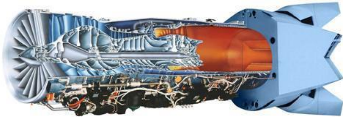
Figure D-3. F-119 Engine Cutaway (Pratt and Whitney, 2002)
