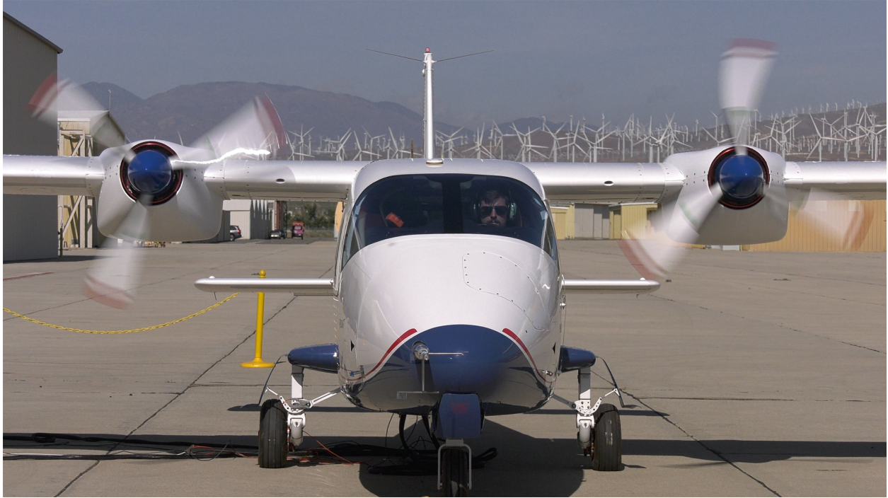
Figure 3. Mod 2, the Tecnam P2006T Airplane with Electric Cruise Motors.
