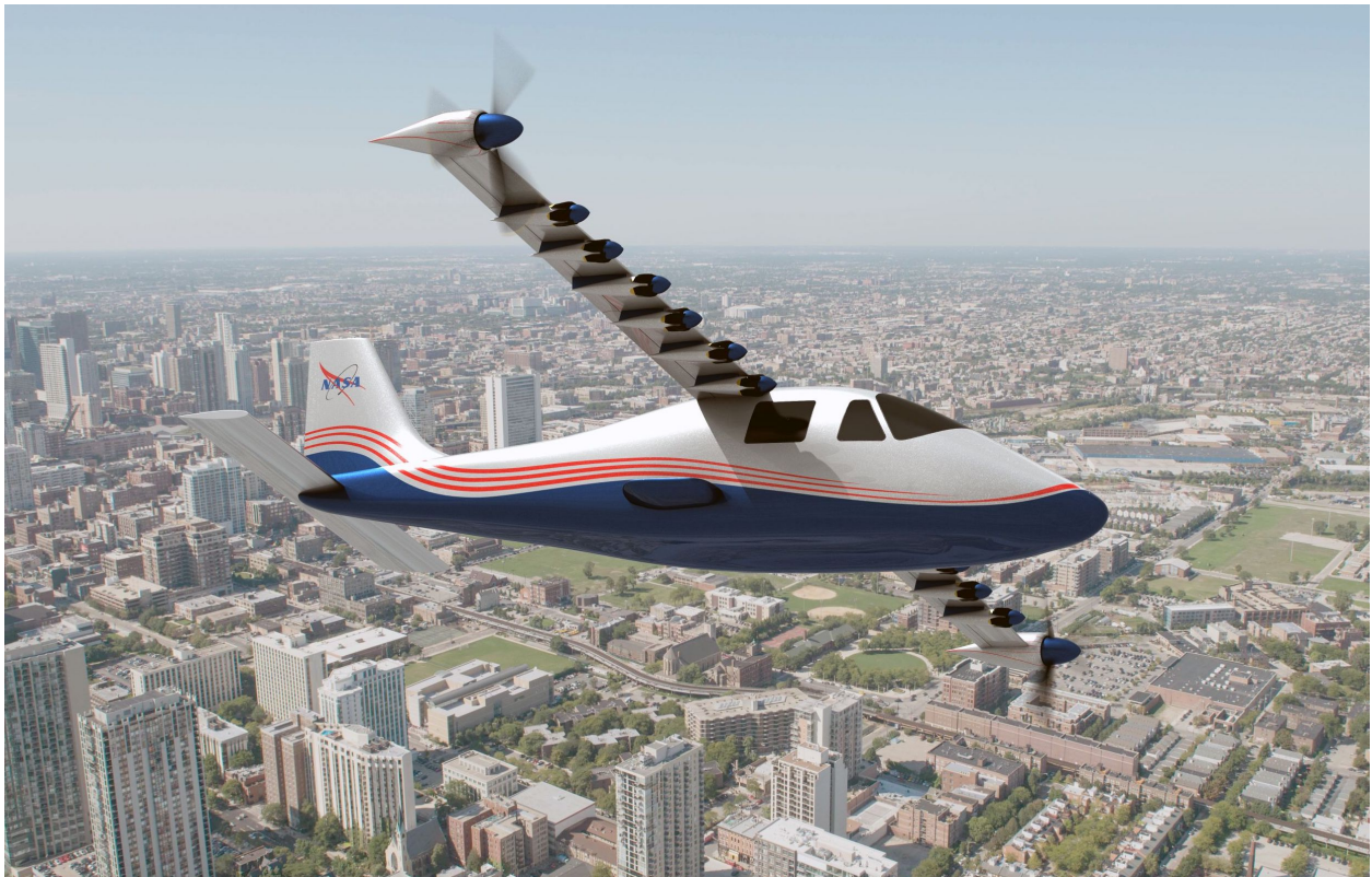
Figure 4. Concept Image of Mod 3, the X-57 Maxwell Airplane with Cruise Propellers Operating and High-Lift Propellers Stowed.
