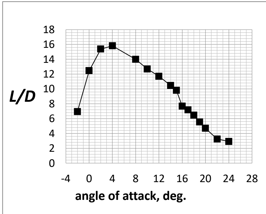
(a) Lift to Drag Ratio as a Function of Angle of Attack
