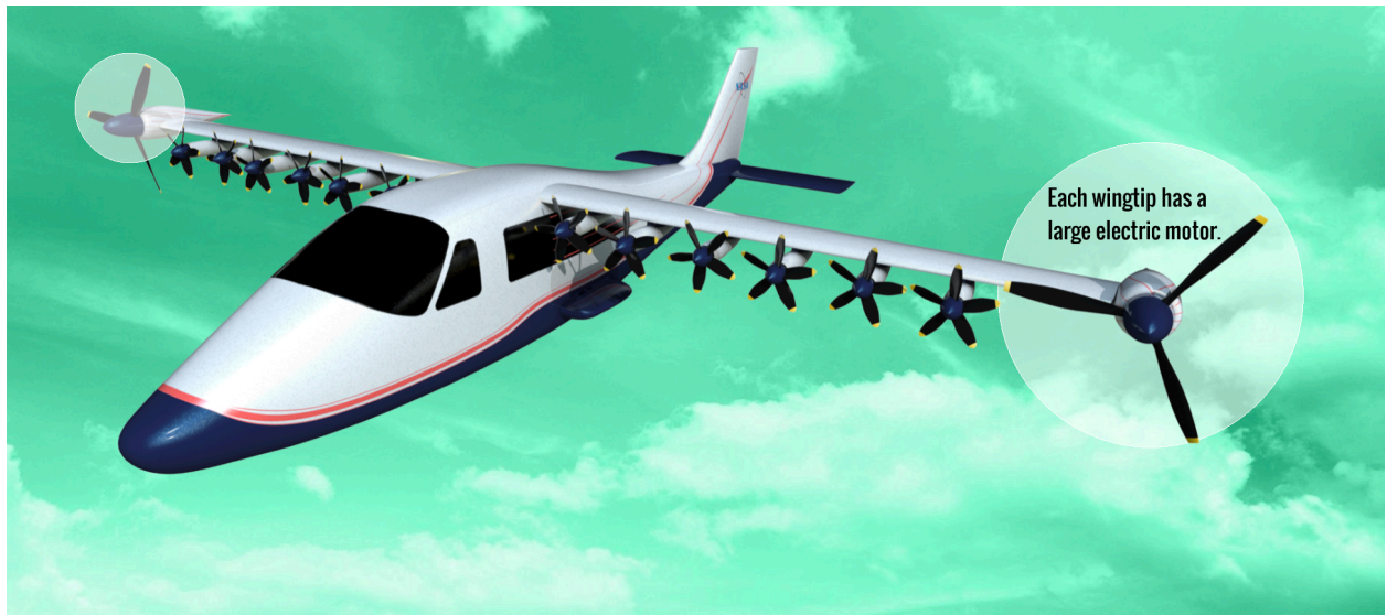
Figure 5. Concept Image of Mod 4, the X-57 Maxwell Airplane with Cruise Propellers and High-Lift Propellers Operating.
