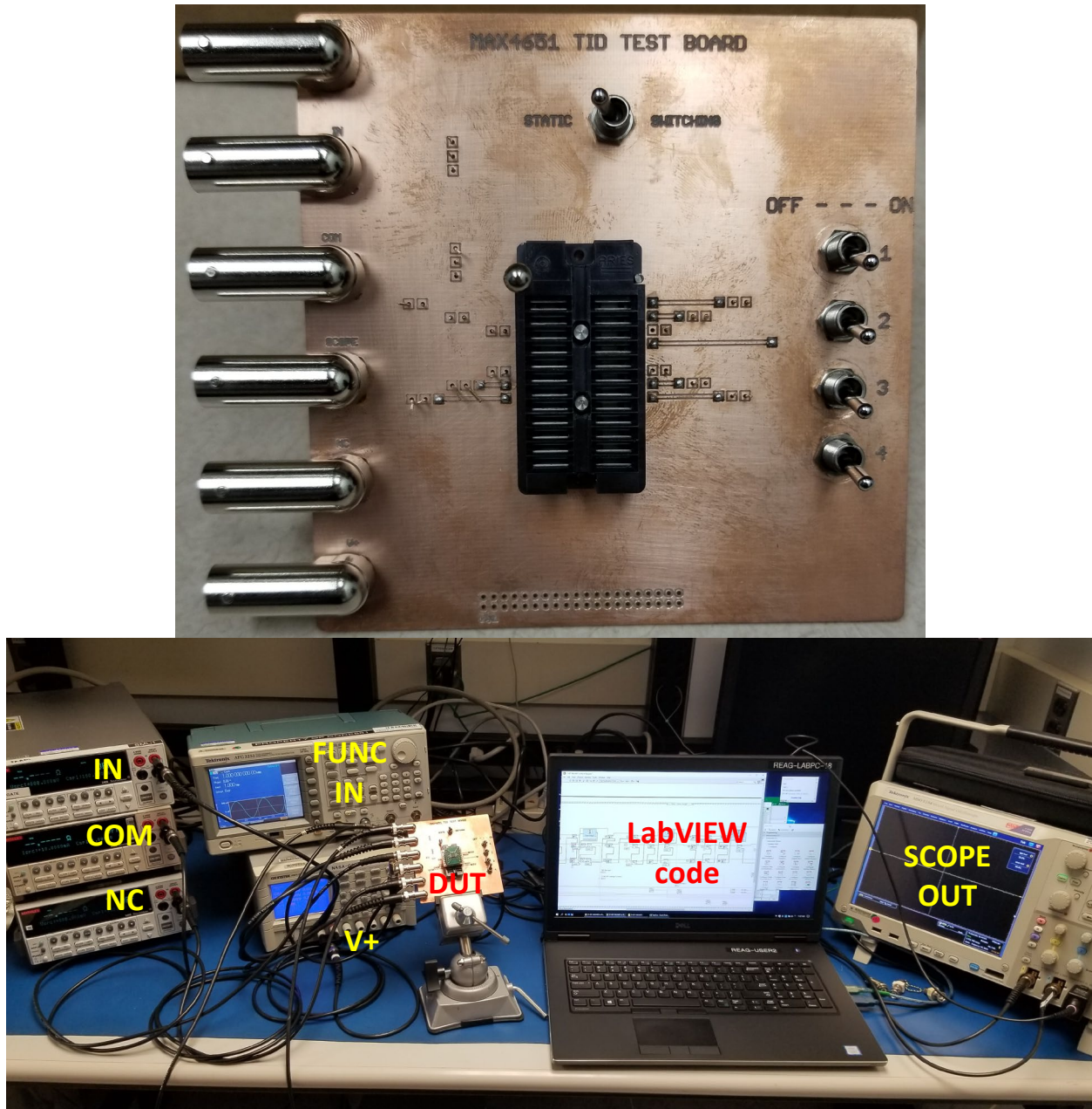
Fig. 2: Picture of electrical test board (top) and test bench (bottom)
