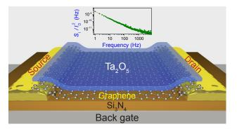
Schematic of graphene devices including back-gate, graphene, dielectric layers (Si<sub>3</sub>N<sub>4</sub>, Ta<sub>2</sub>O<sub>5</sub>), and 1/f noise.
