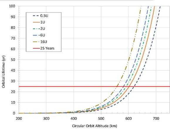
In addition to the 25-year limit, CubeSat developers and operators should consider the functional requirements for collision avoidance when deploying above ~550km
