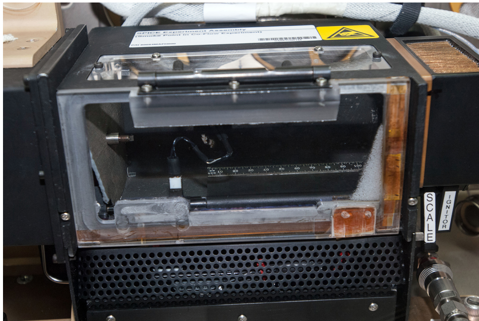
Figure C.1.—Repaired duct door seal and interlocks, showing bubbled lower right corner.
