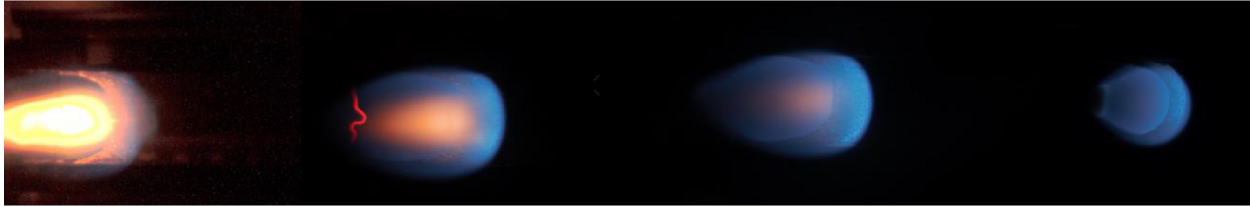
Figure 5.3.—M17 still images at different flow velocities. Last image is just before extinction as flow is turned off.
