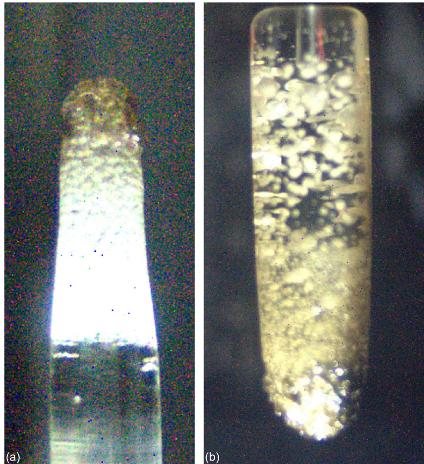
Figure 4.5.—Polymethylmethacrylate rod bubble layers (a) opposed and (b) concurrent.
