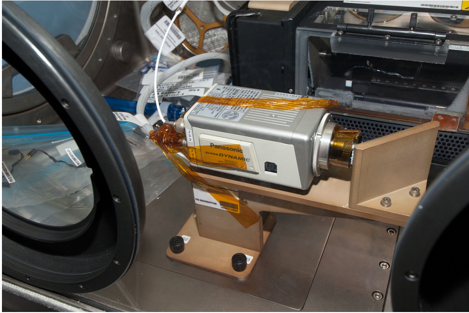
Figure C.2.—Video cable repair and strain relief.
