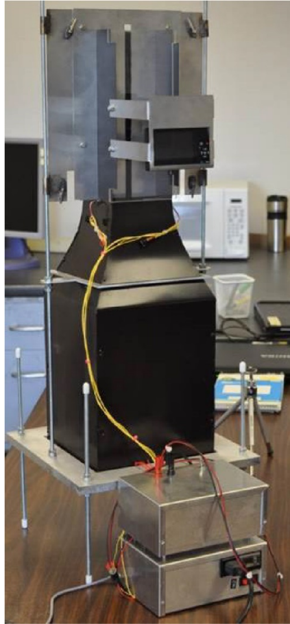
Figure 2.4.—San Diego State University flame tunnel has same dimensions as Hirano tunnel.
