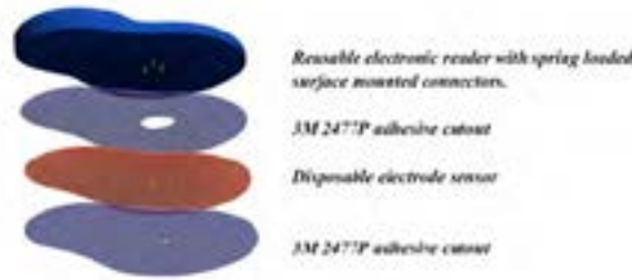
Fig. 1 Stackup of layers in AstroSense sensor.
