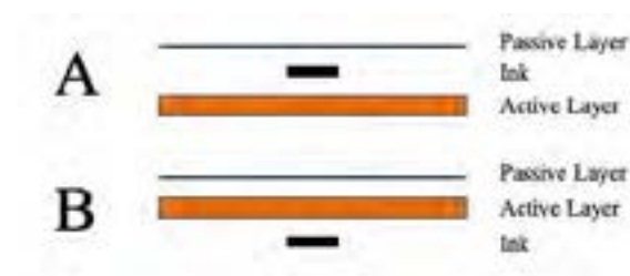
Fig. 13 Orders of lamination of active layer (SMP) with passive layer (Mylar or Kapton) and location of ink. A. Ink between active and passive layers. B. Ink on opposite side of active layer as passive layer.
