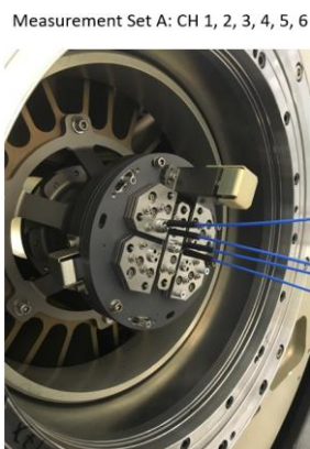
Figure 8. GEDI Focal plane plate assembly with fibers during plate scale measurement.
