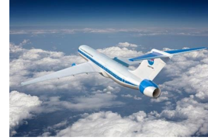
NASA Single-aisle Turboelectric AiRCraft with Aft Boundary Layer propulsor (STARC-ABL) Concept Aircraft
