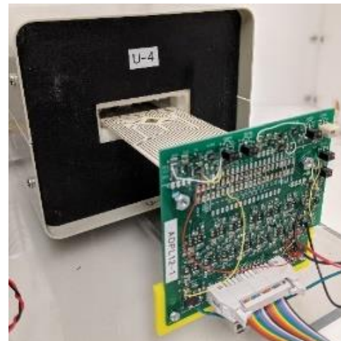
Fig. 4. Illustration of SiC chip compact oven electrical connection and insertion hardware.
