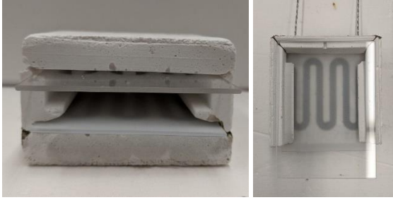
Fig. 7: Side view and bottom view of the custom ceramic heater cavity assembly with COTS quartz plate inserts for reducing particle fallout.
