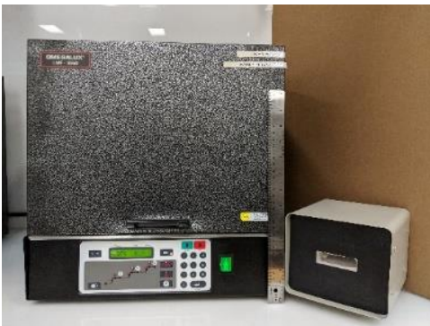
Fig. 2: Oven Size Comparison of COTS oven (left) and compact oven heating enclosure
