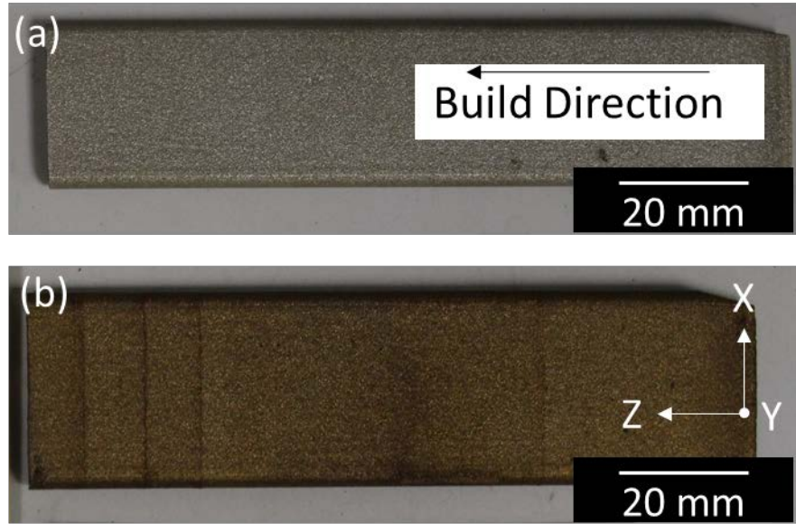
Fig. 1: An example of an (a) as-fabricated metallography bar and (b) a fully heat-treated metallography bar. Z denotes the build direction.
