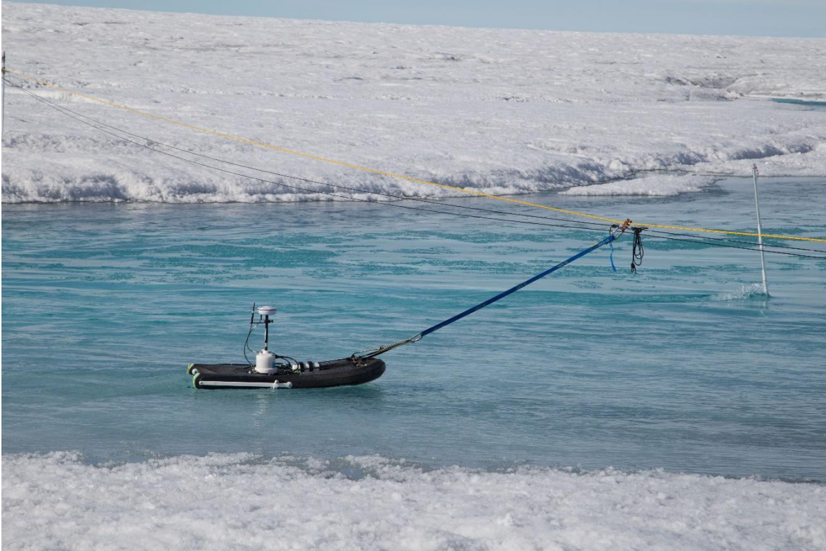
757 Figure S3. Photograph 3 of ADCP discharge monitoring site. Close up photograph of 758 the SonTek River Surveyor® M9 ADCP mounted on a SonTek HydroBoard II. 759 760
