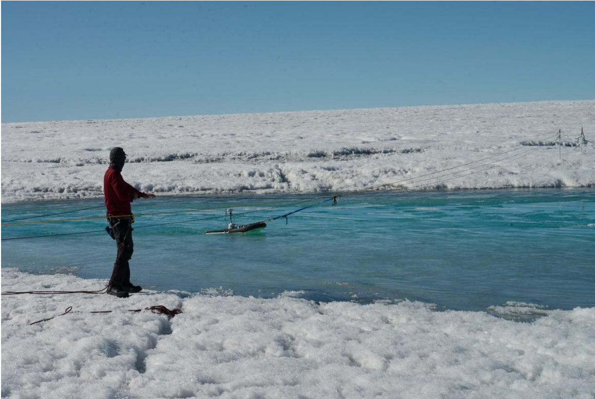
741 Figure S1. Photograph 1 of ADCP discharge monitoring site. A SonTek River Surveyor® 742 M9 Acoustic Doppler Current Profiler (ADCP) mounted on a SonTek HydroBoard II being 743 ferried across the Rio Behar supraglacial river channel cross-section in southwest 744 Greenland (location 67.050°N, -49.018°W). The ADCP and hydroboard are tethered to a 745 specialized bank-operated cableway developed by the field team for deployment on ice 746 surfaces. Data relay is wireless (radio frequency). A total of 847 ADCP profiles were 747 collected every hour for one week (5-13 July 2016). For a time-lapse camera video 748 showing measurement collections and diurnal discharge cycles throughout the week see 749 Dataset S7, Dataset S8, Dataset S9.
