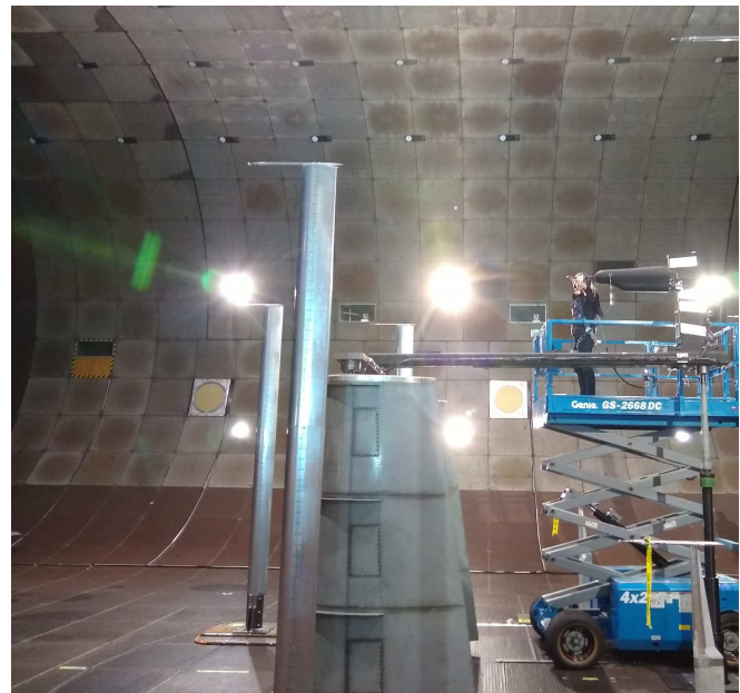
Figure 5. Pistol Reflection Test shooter pointing into the wind at the propeller hub center of the AART propeller.
