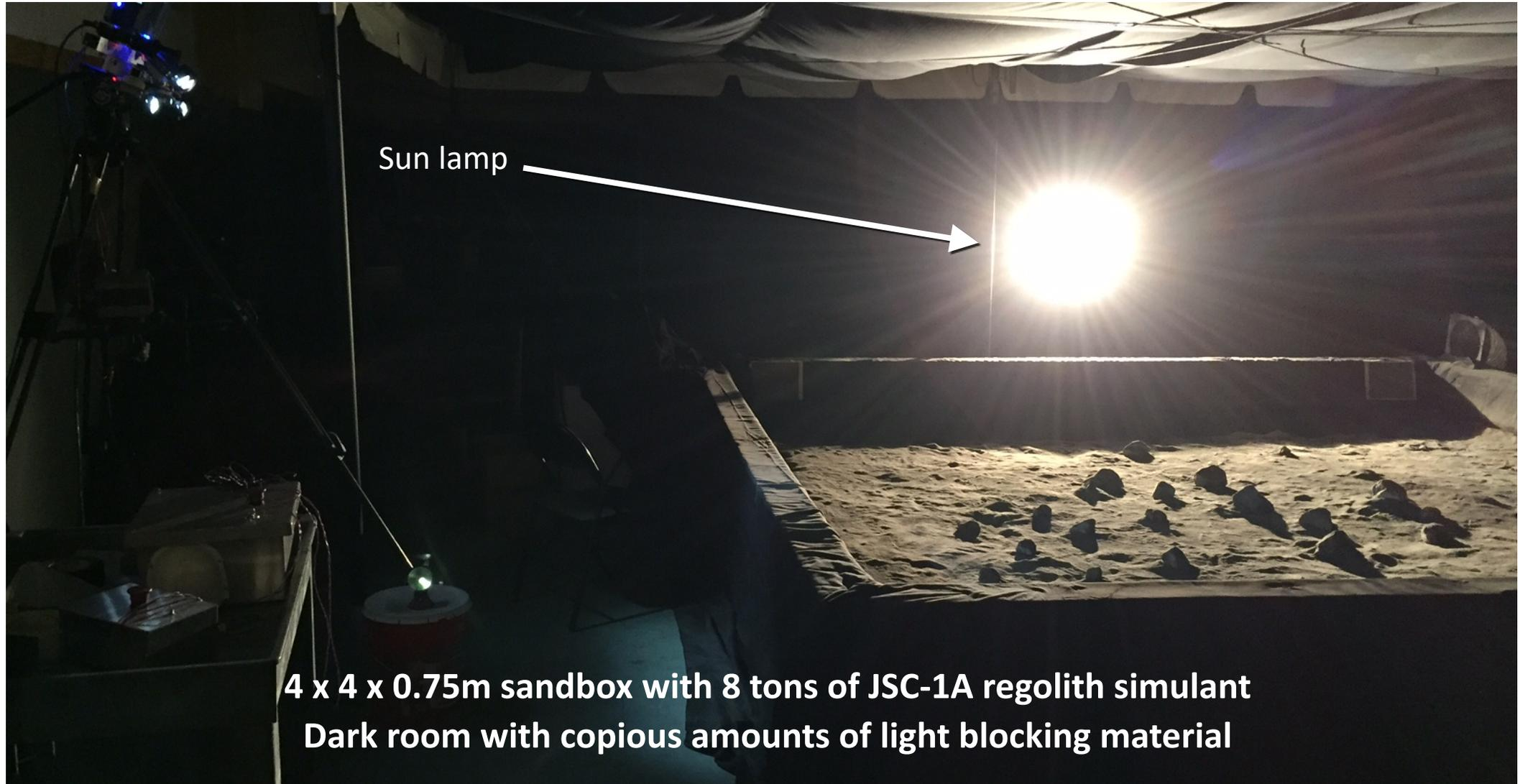
**4 x 4 x 0.75m sandbox with 8 tons of JSC-1A regolith simulant**
