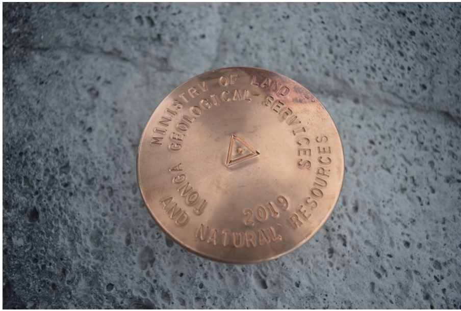
Fig. 3. Geodetic marker installed on HTHH at the request of the Kingdom of Tonga. It reads “Ministry of Land and Natural Resources, Tonga Geological Services, 2019.” Photo Credit: SEA.
