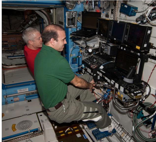
Figure 26. NASA Astronauts Rick Mastracchio and Steve Swanson (ISS Increment 39) Working ISS RWS in the U.S. Lab, with Hand Controllers, Display and Control Panel, and Monitors in View
