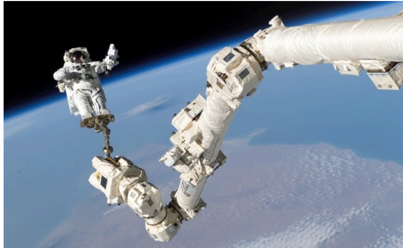
Figure 27. Completing an EVA Activity using the Robotic Arm with a Crewmember on the End Effector
