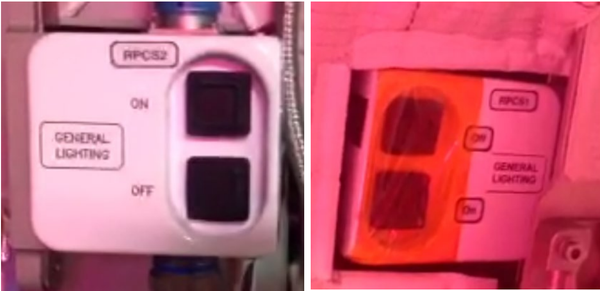
Figure 9. Two Light Switches in the Same Module with Inconsistent Interfaces (Picture from Green et al., 2018)
