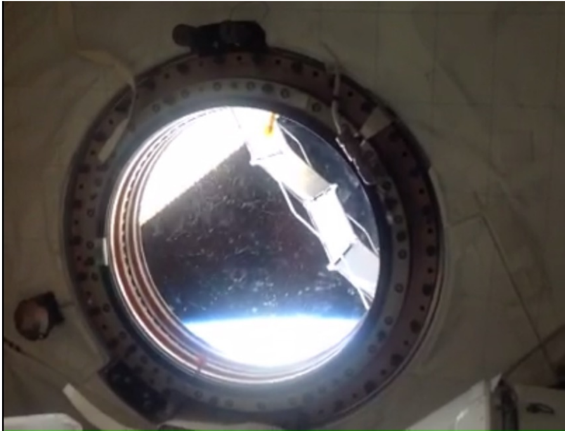
Figure 15, A Screenshot from a Video Showing a Scratch Pane on the ISS Window (Picture from Green et al., 2018)
