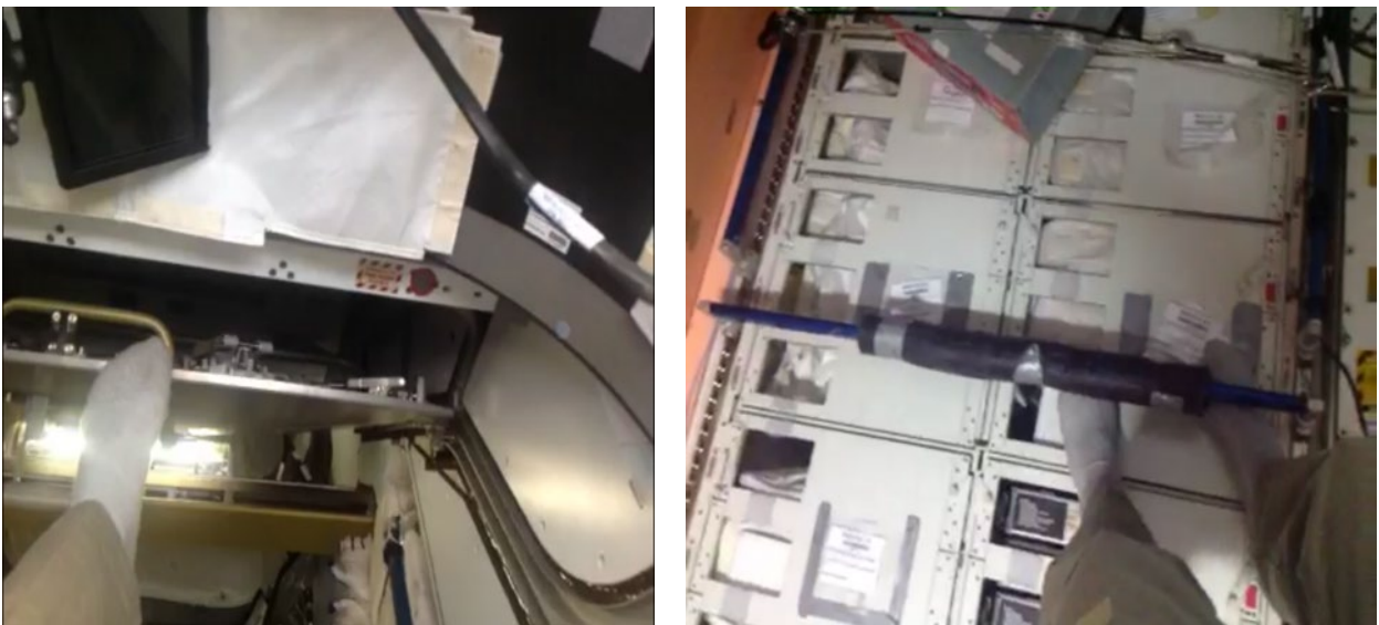
Figure 16. Improved Foot Restraint in the Cupola. The Crewmember is Using the Hatch Opening for Stabilization (Left). Crewmembers Modified this Restraint in the Dining Area to Increase Comfort (Right). (Pictures from Green et al., 2018).
