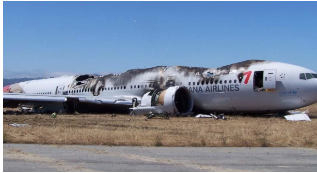
Figure 37. Fire damage to the Fuselage of Asiana Flight 214. (NTSB, 2014b)
