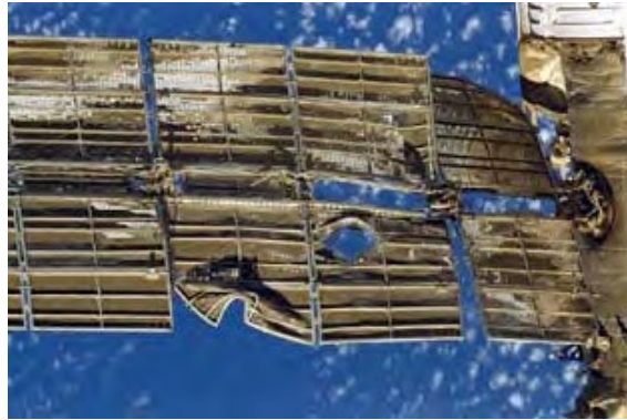
Figure 31. A Mir Solar Array with Damage from a Collision with an Incoming Progress Spacecraft on June 25, 1997
