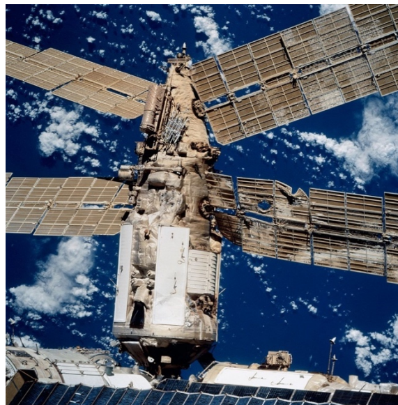
Figure 24. Spektr Module Showing the Damaged Radiator and Solar Array on Mir Space Station
