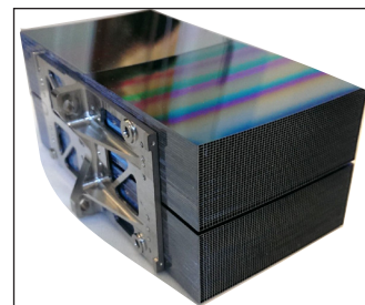
Figure 8 Sample SPO MM with lightweighted mounting structures.
