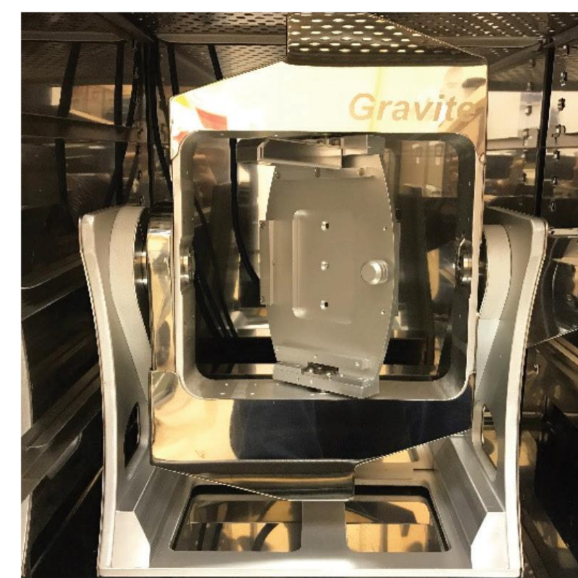
Figure 1. A 3-D Clinostat, one of the many microgravity simulator devices available at the MSSF.
