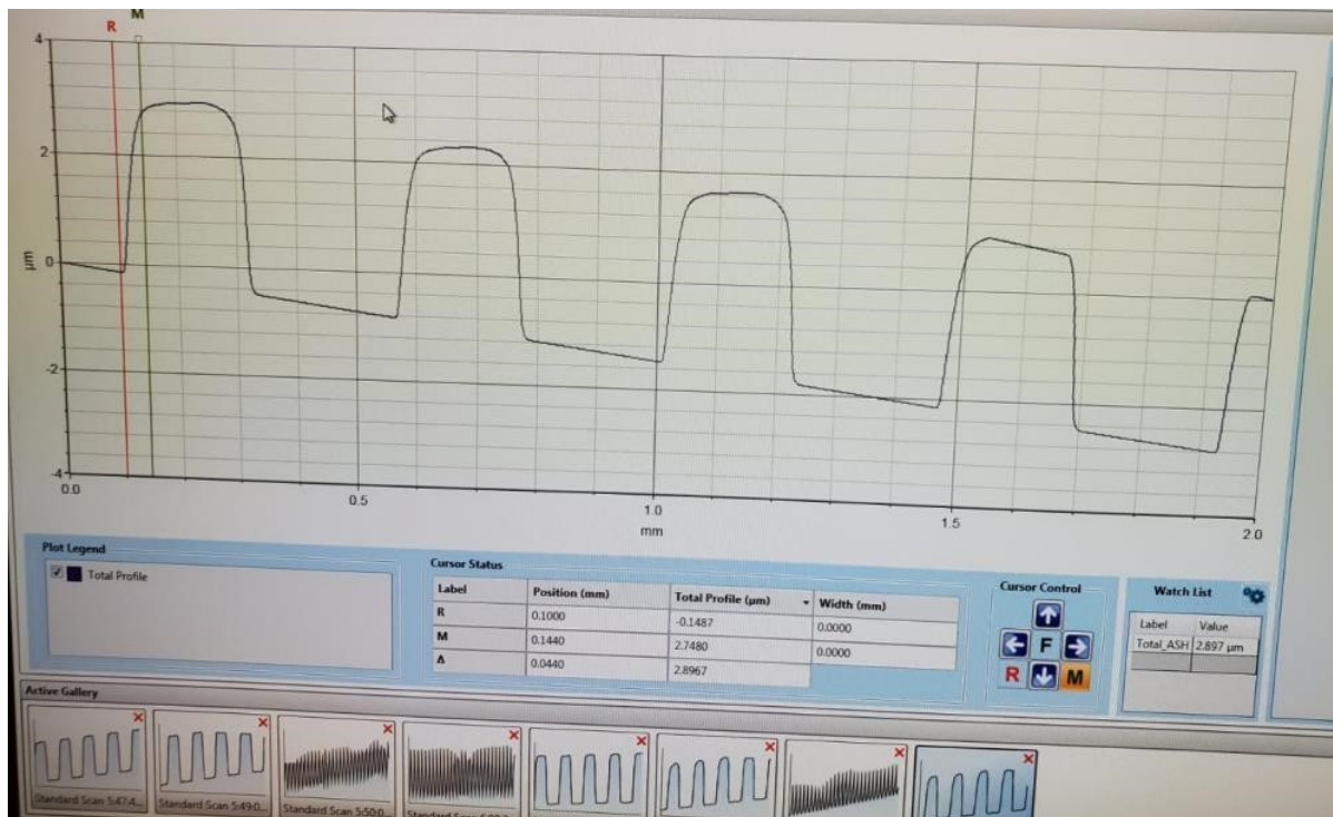
Figure 8. Depth of 230μm gratings on wafer
