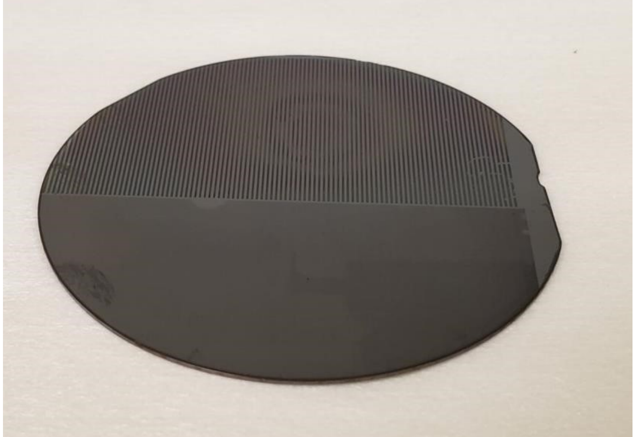
Figure 3. A multi spacing QPM design for silicon wafer
