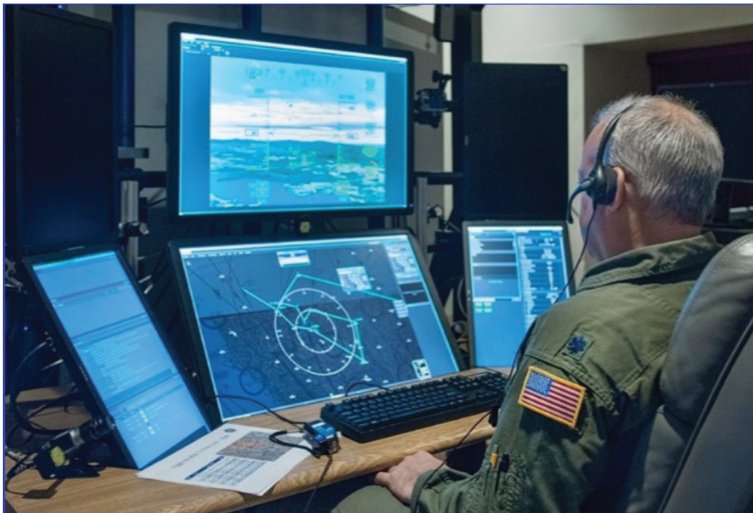
Figure 7. Air Force Research Laboratory's Vigilant Spirit Pilot Station, integrated with Detect and Avoid (DAA) alerting and suggestive guidance. (NASA Ames).
