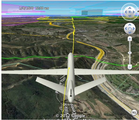
Figure 6. Concept demonstration of a synthetic display to assist the pilot with situational awareness. (Image courtesy of Mosaic ATM).
