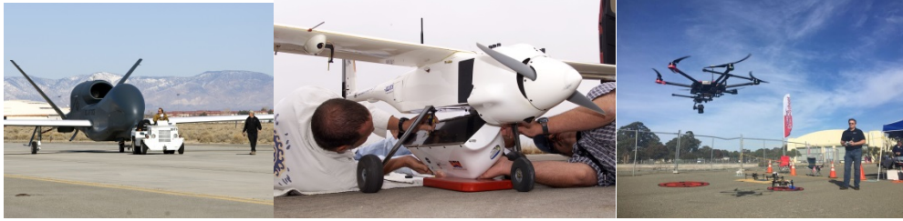
Figure 1. The diversity of unmanned aircraft. From left to right: The 14,600kg Global Hawk (Image courtesy Northrop Grumman); the 20 kg RnR APV3 (NASA image); and the 9.5 kg DJI Matrice M600 hexacopter (Image courtesy Werner von Stein, SF Droneschool).
