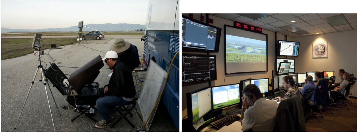
Figure 4. Remote Pilot Stations (RPS) range from commercial off-the-shelf laptops, to purpose-built facilities. Shown here is the RPS for the 7 kg MLB Bat, with car-top launcher visible in background (NASA image); and the control room for NASA's Global Hawk Unmanned Aircraft at NASA Armstrong Flight Research Center. (NASA photo: Tony Landis.)
