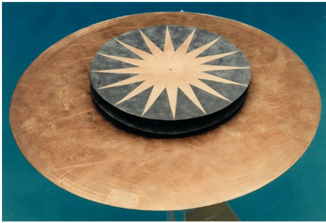
Fig. 8 Sixteen-element tapered slot circular array above a ground plane and with a parasitic array above
