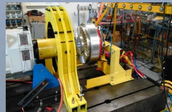
OSU MW motor connected to electric load machine
