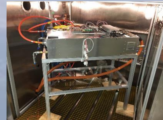
Gen3 inverter in altitude chamber
